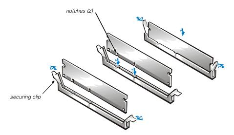
Figure 8-6. Installing a Memory Module
